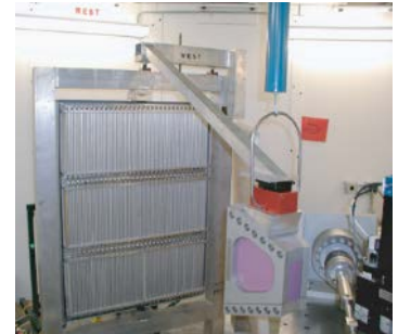
"Short" radial collimator supported between load frame and detector.
