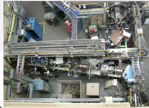
Top view of 750 keV H+ LEBT (lower) and H- LEBT (top) merging to right before DTL located in Sec J.
