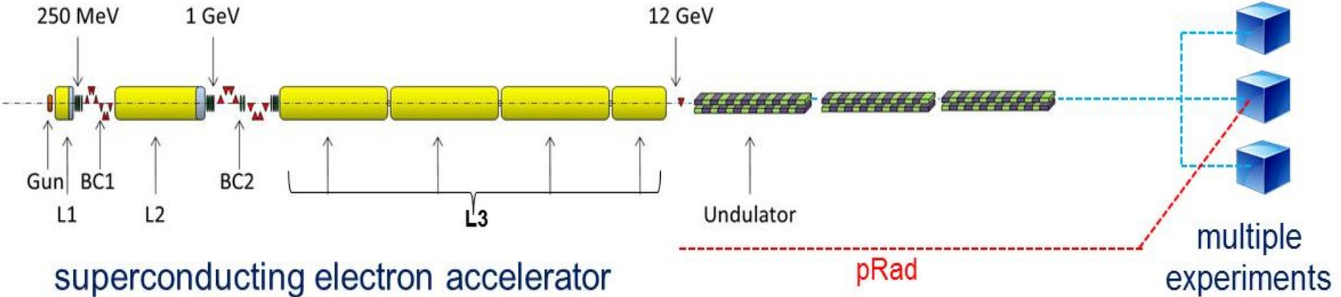
The pre-conceptual reference consists of a 12-GeV electron linac feeding a 42 keV XFEL. Located on the the LANSCE mesa it can leverage the capabilities of the existing proton/neutron facilities.
