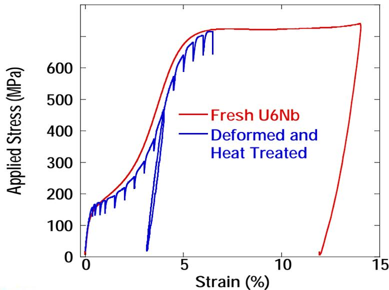
Measurements on predeformed U6Nb demonstrate that microstructure (and thus ductility) is recovered by a simple heat treatment to 800C.
